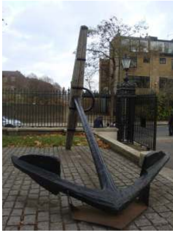
FIGURA 7.11 – ANCLA TIPO OLD ADMIRALTY LONGSHANK .
